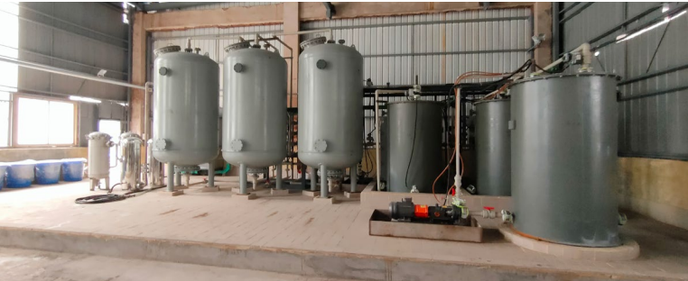
Research and Application of Lithium Sulfate Solution Resin-Based Calcium Removal Equipment and Process Technology
